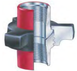
Fig 400 Union cold working pressure 1"- 4" 4,000PSI (276bar) 5"-12" 2,500PSI (172bar)
